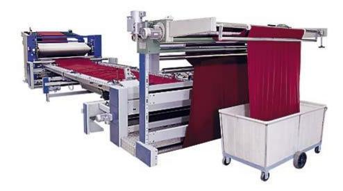
Compaction is a mechanical finish in which the length of the fabric is reduced by compressing the structure of the fabric. The fabric is more likely to shrink because of its structure. Fabric structures that have more open style have greater propensity to shrink. Compaction helps to avoid this.
