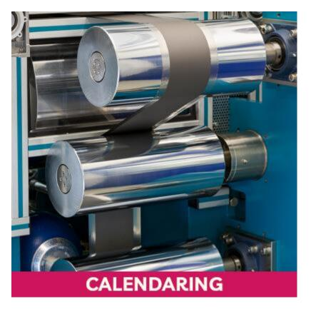
When a fabric is wet processed and dried, it will be in its least lustrous state. The surface will be rough due to the presence of highly crimped and wavy threads. In order to solve this problem, the fabric is passed in between two rollers or bawls of a machine called as a 'Calendar'. Hence the process is called as calendaring.
