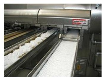
During processes like spinning or weaving, the chances of fabric undergoing distortions in fabric structure, designs and also uneven shrinkage is higher. In order avoid this, setting is implemented. Setting stabilizes the woven structure of the fabric in a regular and permanent manner by relaxing the stresses. The
